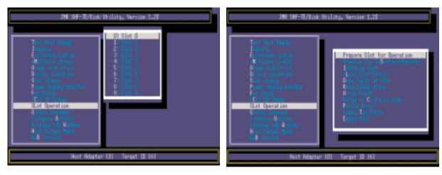
The *Global Command Screen*, has several flags that may be set that affect the entire enclosure, not just a particular slot. The first two commands are important to unit operation and the rest of the flags are mainly used for test purposes. *Clear Global Errors* will clear any enclosure error flags that have been set
